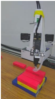
Figure 6.20: The suction cup end-effector is picking the 1 st rectangular box (red) from the starting picking coordinate
