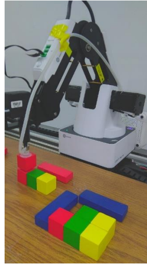
Figure 6.15 After placing the 1st row of cubes, the end-effector is placing the red cube on another red cube placed at the beginning
