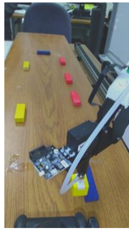
Figure 6.53 When the user gives a voice command 'Water', the suction cup end-effector reaches the predefined location of the water to grab it
