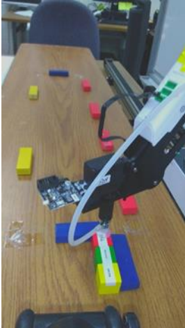
Figure 6.417 When the user gives a voice command 'Tea', the suction cup end-effector reaches to the predefined location of Tea to grab it
