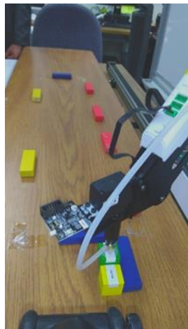
Figure 6.52 When the user gives a voice command 'Coffee', the suction cup end-effector reaches to the predefined location of the coffee to grab it
