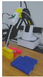
Figure 6.23: The suction cup end-effector is stacking the last yellow rectangular box on other yellow boxes.
