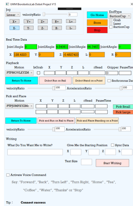
Figure 5.1 Windows application for controlling Dobot developed with C# programming language
