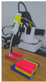
Figure 6.21: The suction cup end-effector is placing the 1 st rectangular box (red) to the starting placing coordinate
