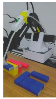
Figure 6.24: The suction cup end-effector is starting to place blue boxes adjacent to the yellow box columns.
