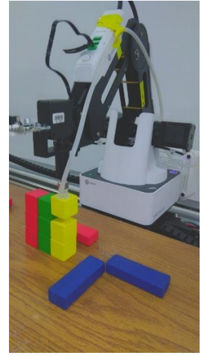
Figure 6.16 The end-effector stacked all red cubes together, all green cubes together and now stacking the last yellow cube
