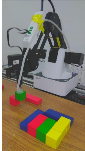
Figure 6.14 After picking the 2nd cube (green), the end-effector is placing it to the next available placing position
