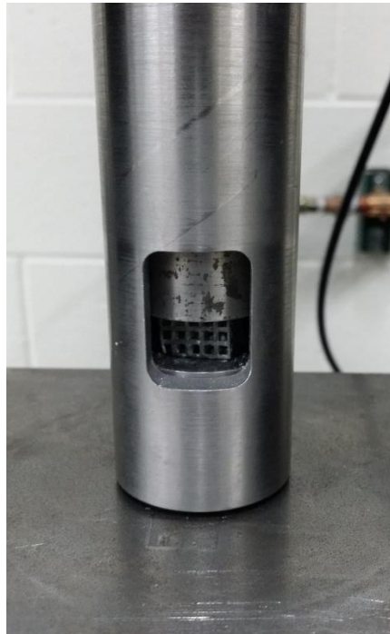
Figure 18: Scaffold in compression testing fixture
