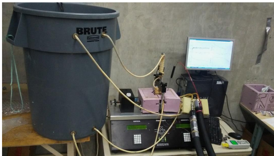
Figure 4-5- Actual modified direct shear test setup, external water bath and water circulation plastic tubes.
