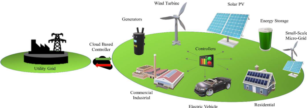
Figure 10: A schematic picture of the energy network including distributed generations.
