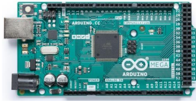
Figure 67. Example of Arduino Mega 2560 microcontroller
