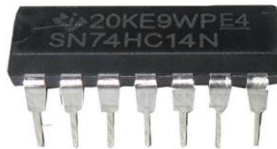
Figure 69. Schmitt trigger inverters 74HC14 IC
