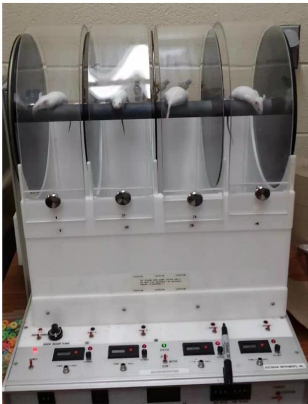
**Figure 46. Mice running on the RotaRod Apparatus** The RotaRod apparatus has individual compartments for each mouse to maintain the animal's focus. The area beneath the rod is enclosed to contain the animals if they fall. The rod is high enough to encourage the animals to stay on the rod, but not so high as to cause injury if they do fall.
