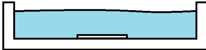
Figure 4.11 – Glass slide submerged in photoresist remover and oriented horizontally during sonication.
