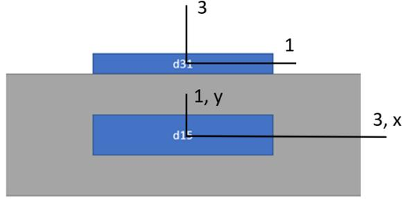
Figure 11:  $d_{31}$  and  $d_{15}$  PZT in aluminum
