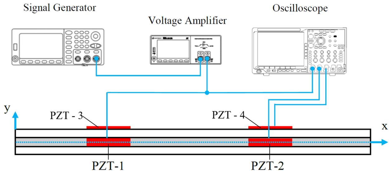
Figure 31: Schematic of experimental setup
