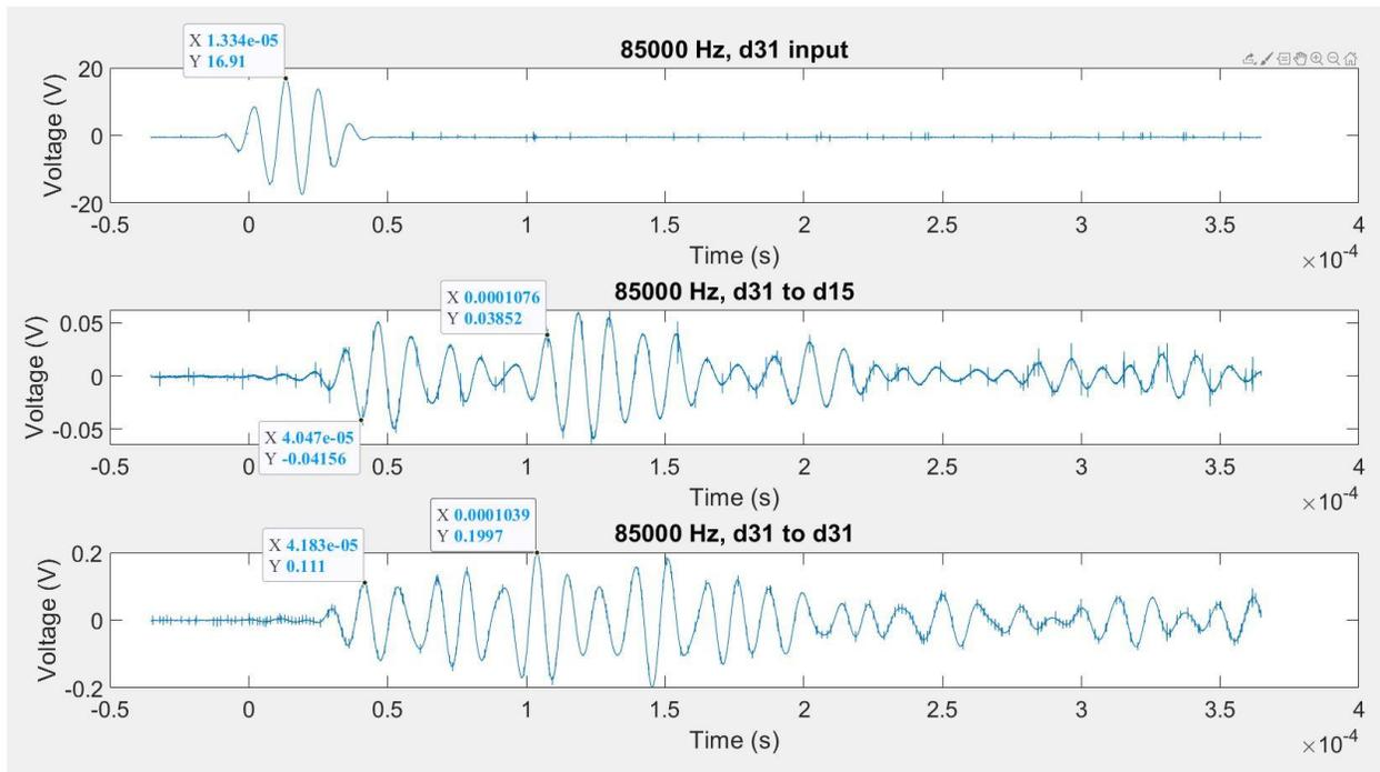
Figure 33:  $d_{31}$  actuation response at 85000 Hz. Aluminum sample.
