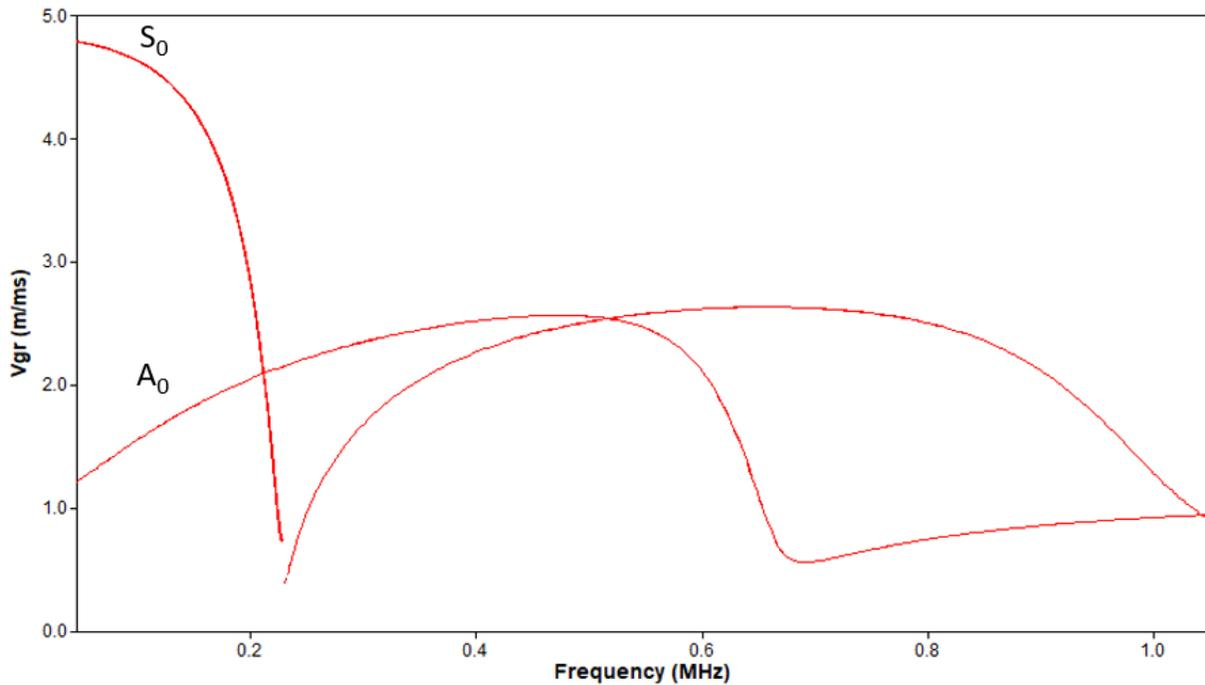
Figure 34: Group velocity curve for aluminum sample
