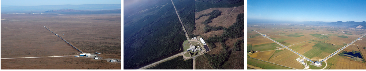
Figure 1.1 Aerial views of the Advanced LIGO and Advanced Virgo detectors. Each of the LIGO detectors have 4 km long arms. The Virgo detector has 3 km long arms. The long arms house a modified Michelson interferometer to detect gravitational waves. From left: LIGO Hanford, LIGO Livingston, and Virgo. Figures credits: www.ligo.org & www.virgo-gw.eu .
