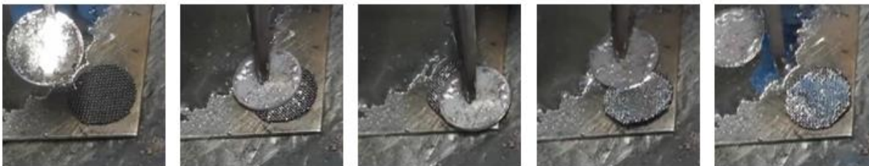
Figure 2. 2 Ironing process lead to a limited/controllable molten Li infusion to single side CFF. 41
