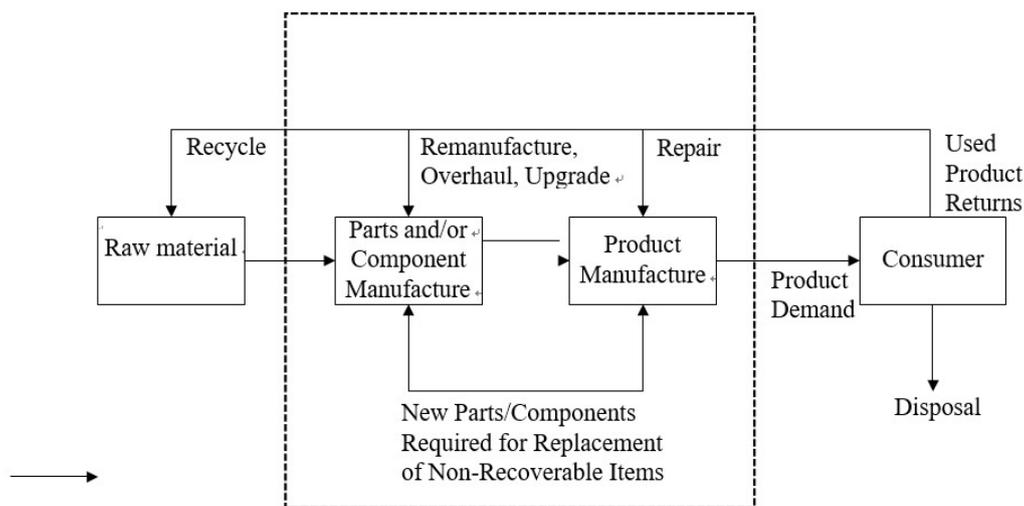
Figure 2.1: Recoverable manufacturing system (Guide et al., 2000).
