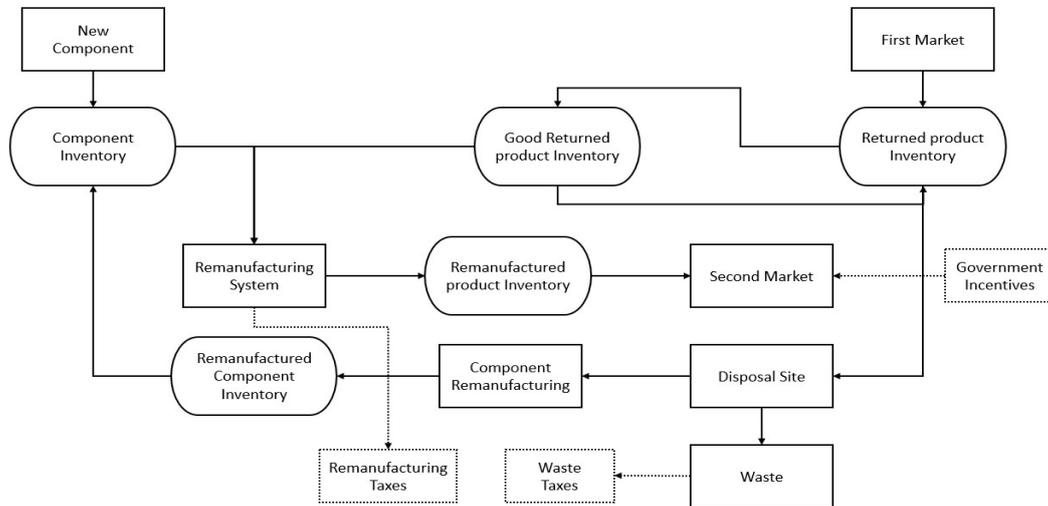
Figure 3.1: Conceptual framework of remanufacturing system, adopted from (Kim et al., 2006).
