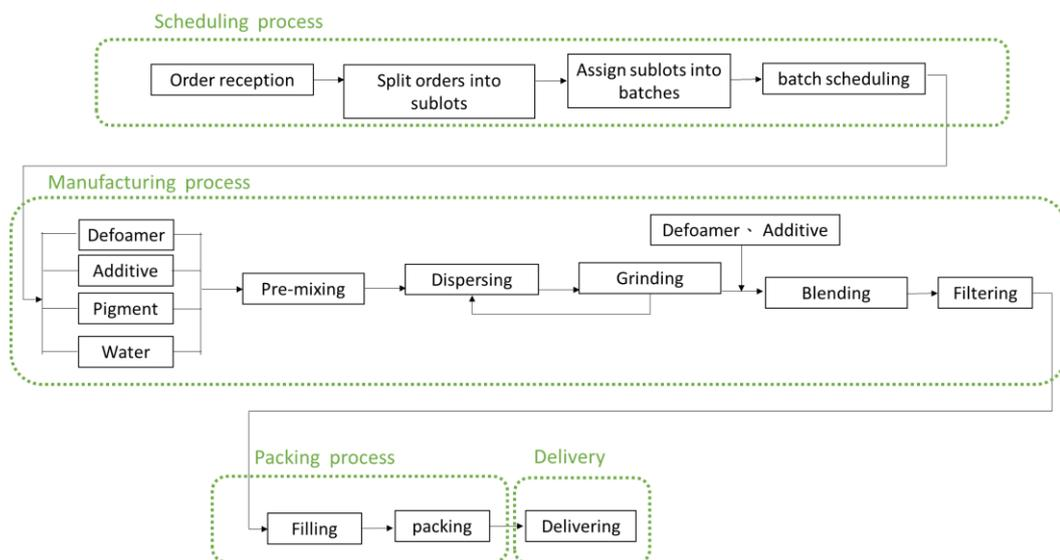
Figure 4 Overall paint production process. Source from: San Nopco<sup>5</sup>
