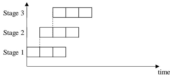
Figure 6 Process batch not equal to transfer batch
