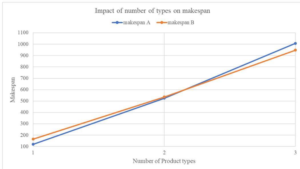
Figure 23 Makespan under different number of product types
