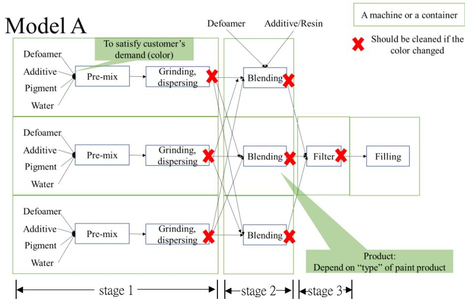
Figure 7 Illustration manufacturing process of model A
