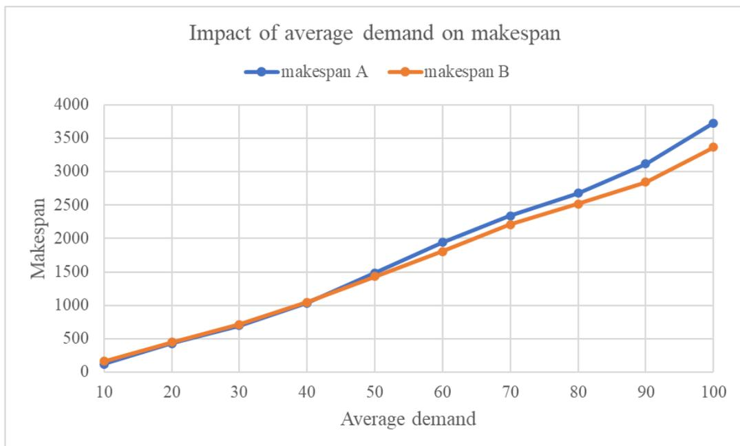
Figure 20 Makespan under different average demand
