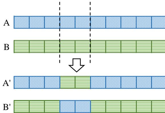
Figure 11 Two-point crossover mechanism
