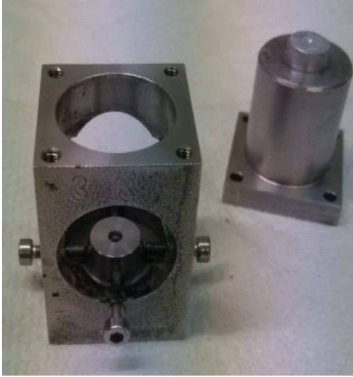
(a) Centering and aligning the seat to place the diamond anvils. Note this is not the DAC.
