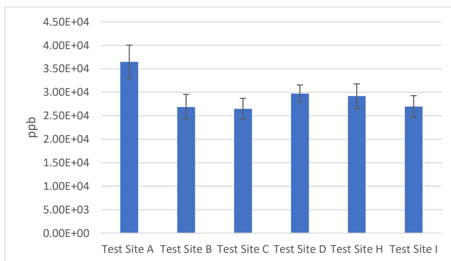
Figure 47. Comparison of Ga abundance in industrial effluent samples. Error bars represent the Student's t value at the 95% confidence interval. (n = 3)
