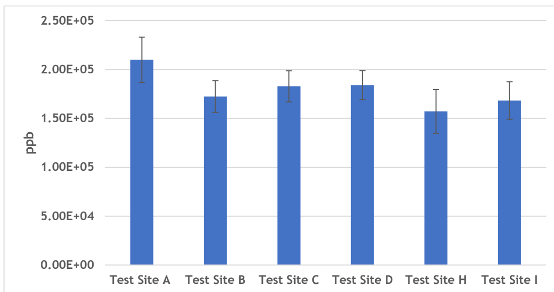
Figure 48. Comparison of Ba abundance in industrial effluent samples. Error bars represent the Student's t value at the 95% confidence interval. (n = 3)
