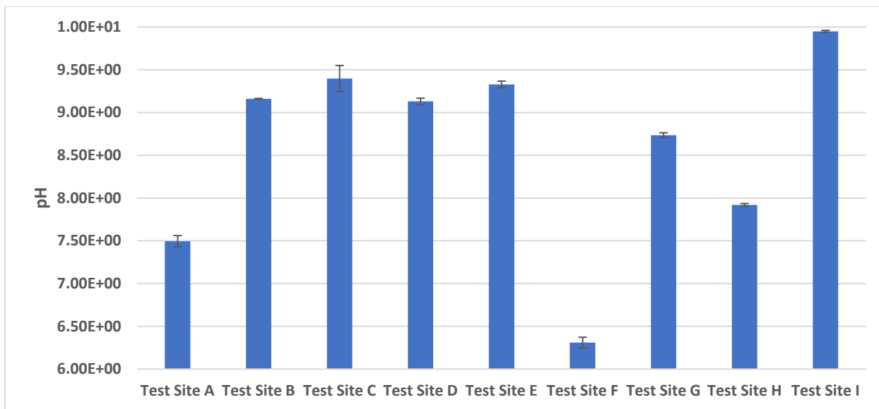
Figure 26. Raw Sample pH (measured directly via pH probe). Error bars represent the Student's t value at the 95% confidence interval (n=3).
