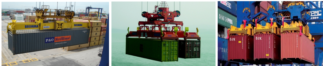
Figure 1.6. Single, double, and triple spreader handling of containers by QCs.
