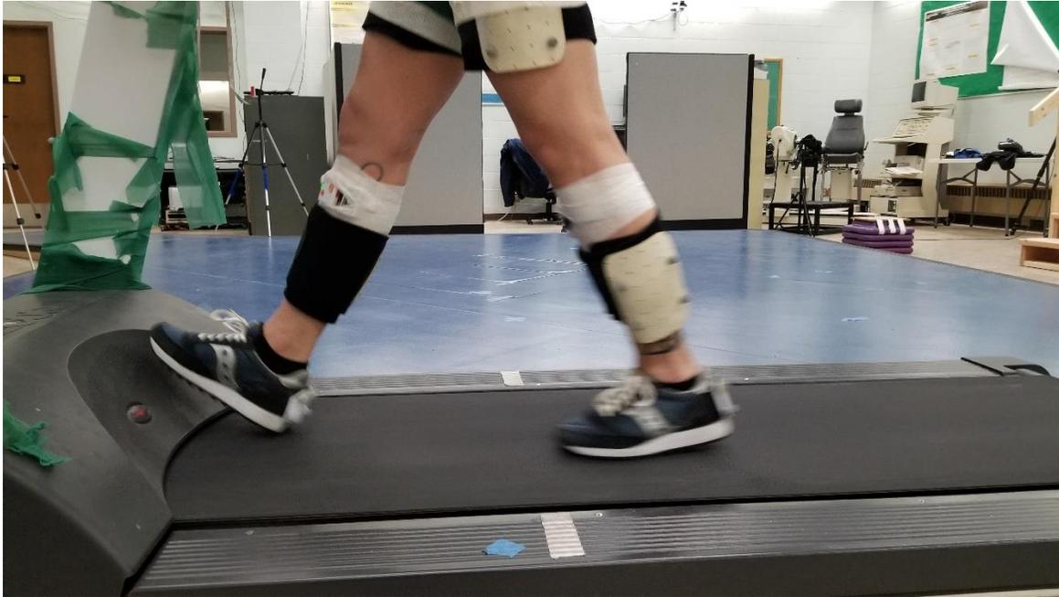
*Figure 1.* Experimental setup following standing calibration for an ACL reconstructed participant. 28 reflective markers were placed on the pelvis and lower extremities. IMUs and accelerometers were placed on the anteromedial aspect of each shank.
