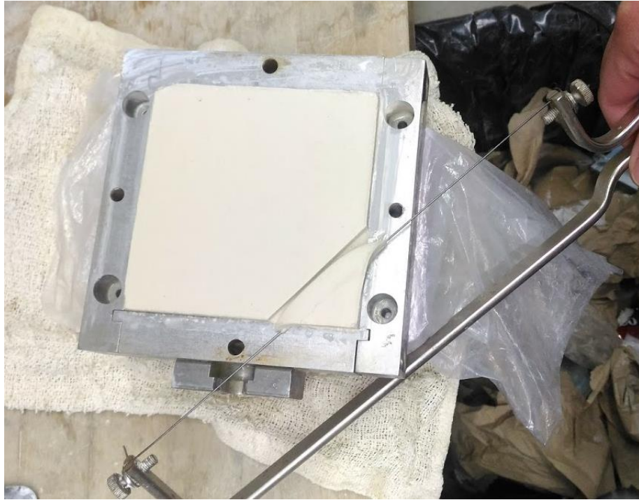
Figure 4-6: Kaolin specimen trimming (for slow soil-concrete direct shear test)
