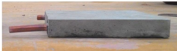
Finish. Ready for testing interface behavior of soil and concrete.
