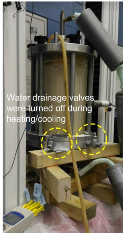
Figure 5-2: The water drainage valves were turned off during heating/cooling
