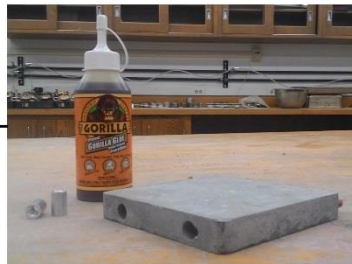
After curing, drilled nut holes in the concrete slab and glued nuts in the holes
