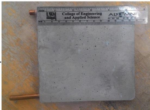
Finish. Ready for testing interface behavior of soil and concrete.
