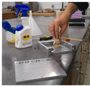
Using WD-40 to lubricate the concrete mold
