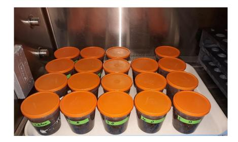
Figure 21. PSM aged in water with three carbonate concentration (0, 0.5, 0.84 g/L) for incubation experiment
