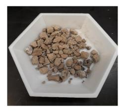
Figure 12. EAF steel slag as a potential PSM
