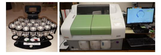
Figure 16. A rack of outflow sample and spectrophotometer used for P analysis
