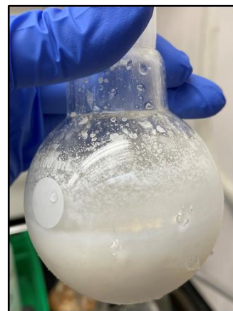
Figure 69. Slurry formation after cold water addition to the DMF trial.
