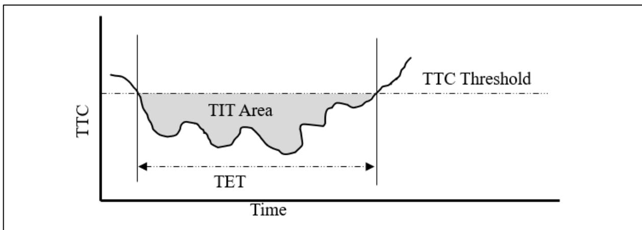
Figure 8 Conceptual diagram of TET and TIT.
