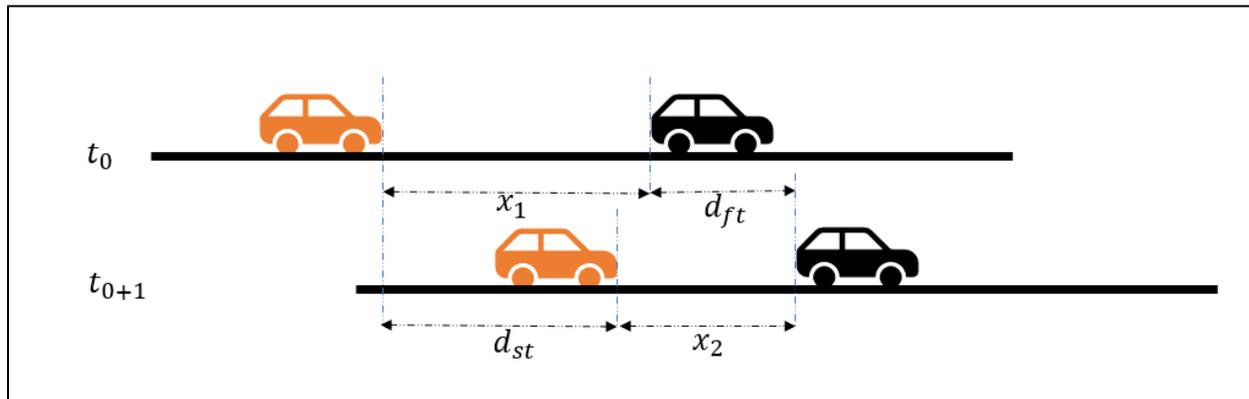
Figure 2 Front vehicle speed calculation from CV.
