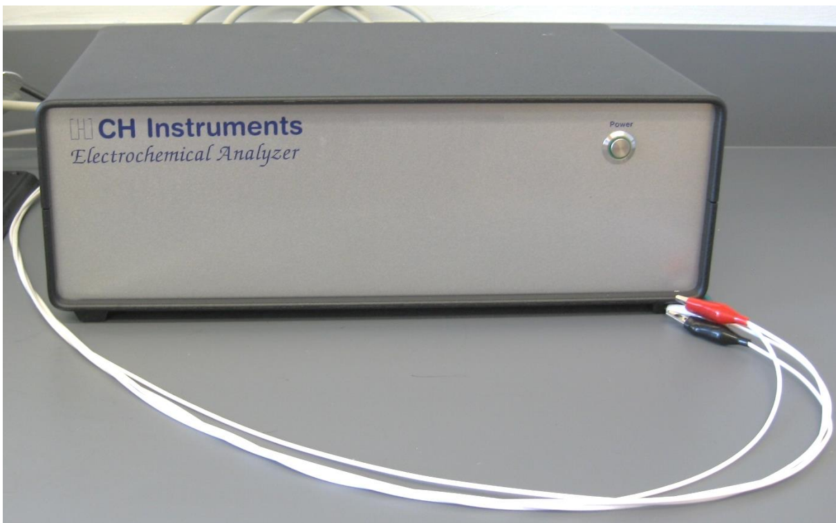
Figure 2: CHI-6012E, a computer-controlled electrochemical analyzer (CHI, USA)
