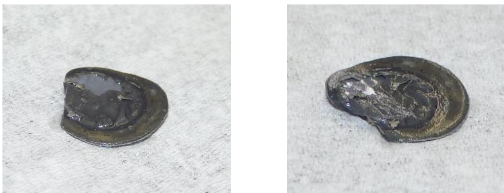
Fig. 4.18 –Representative Images of Delamination of Working Electrodes
