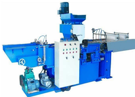
Fig. 2.7 – Representative Image of the Grid Pasting Process [30]
