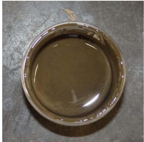
Fig. 3.2 - (a) combination of the dry components of the NAM (b) addition of the PVDF/NMP solution (c) result of the mixing of PVDF/NMP solution and dry components (d) result of mixing the remainder of NMP to PVDF/NMP solution and dry components
