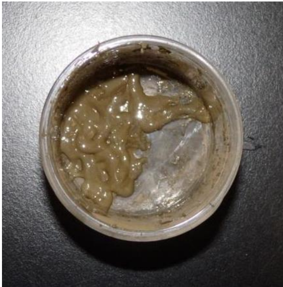
Fig. 3.2 - (a) combination of the dry components of the NAM (b) addition of the PVDF/NMP solution (c) result of the mixing of PVDF/NMP solution and dry components (d) result of mixing the remainder of NMP to PVDF/NMP solution and dry components
