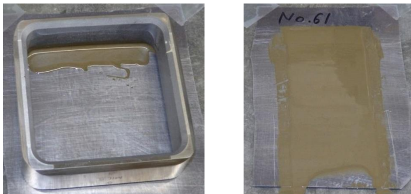
Fig. 3.6 – (a) paste from Fig. was transferred to the 1-8 mils 8 path applicator (b) result of the NAM applied to the abraded Pb foil
