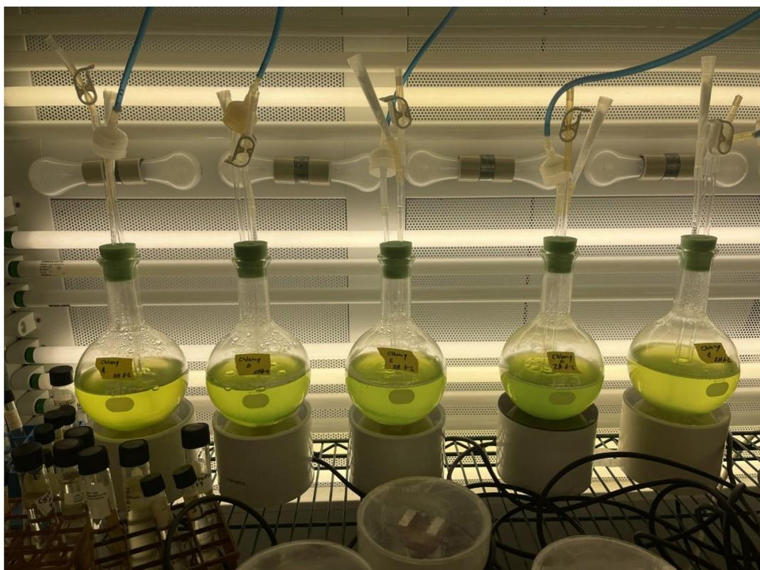
**Figure 2:** Image of sub-culture for high density PFOS removal experiment in the growth chamber with bubbling air (filtered), sampling and exhaust ports.
