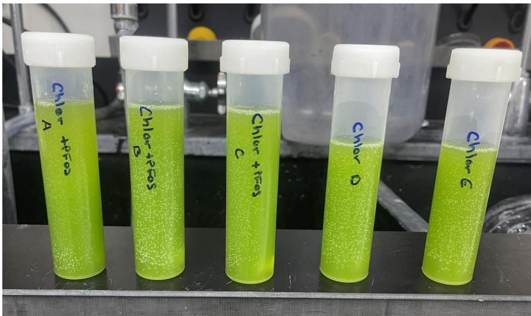
**Figure 3:** Example 60 mL PP tubes with algal cells. Tubes labeled A-C contain PFOS, tubes labeled D and E are for DOC measurements.
