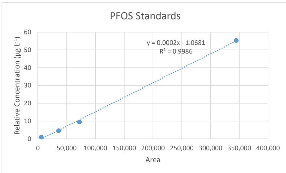
**Figure 6:** Calibration curve for target PFOS detection.
