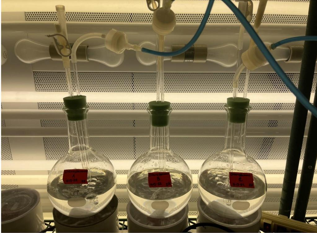
**Figure 1:** Image of algae growth 1-liter round flask set up with bubbling air (filtered), sampling and exhaust ports.
