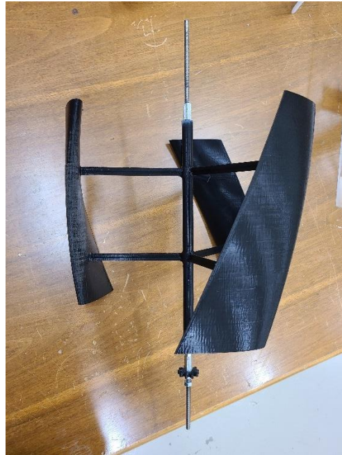
FIGURE 6: MODEL OF THE STRAIGHT H-TYPE TURBINE FOR WIND TUNNEL EXPERIMENTS
