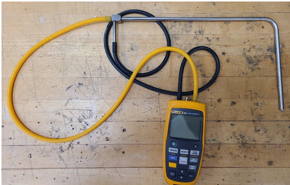
FIGURE 19: IMAGE OF AIRFLOW METER WITH PITOT TUBE ATTACHED
