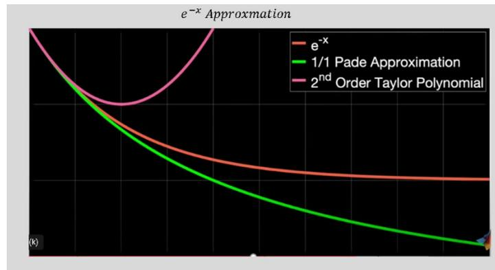
Figure 3-13 Comparison of two methods of time delay approximation
