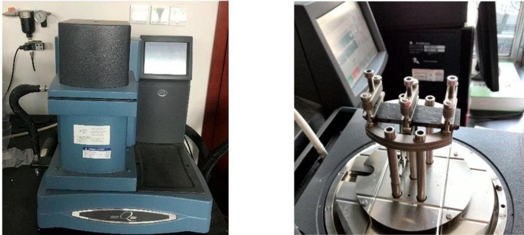
**Figure 3.24: DMA Machine and Cantilever Clamp (Wang, Wang et al. 2022)**
