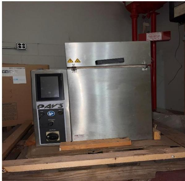
**Figure 3.14: Pressure Aging Vessel (PAV)**
