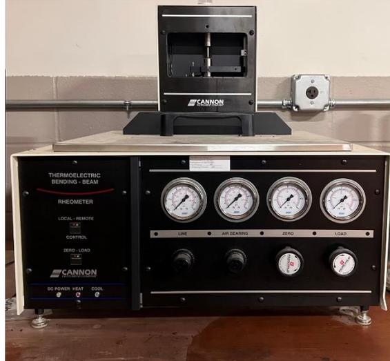
**Figure 3.23: Bending Beam Rheometer**
