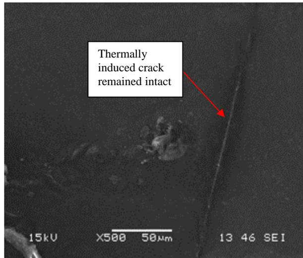
**Figure 4.2: Thermally-induced cracks in limestone-based mastics**
