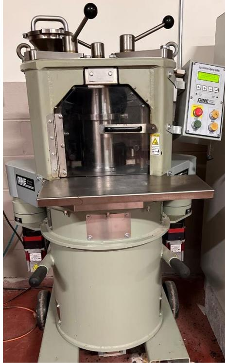
**Figure 3.27: Superpave® Gyratory Compactor**
