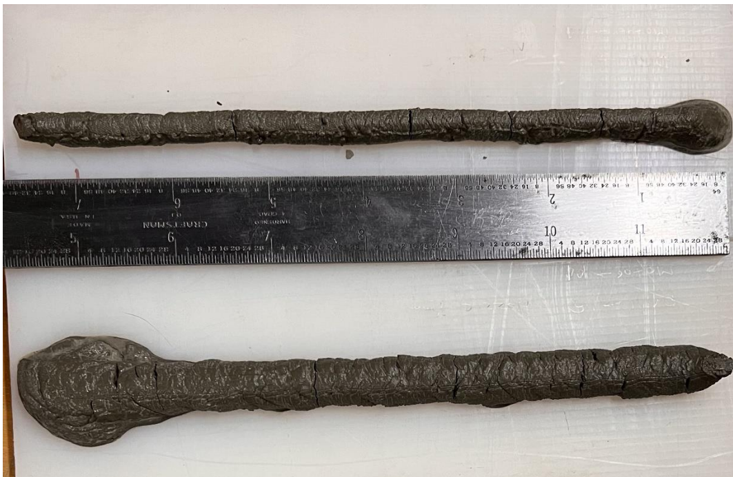
Figure 3-10: Cracks of initial cement prints after 4 hours of lab exposure
