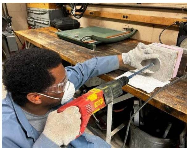
Figure 9 Sampling of Concrete powder from salt ponding slabs with hammer drill
