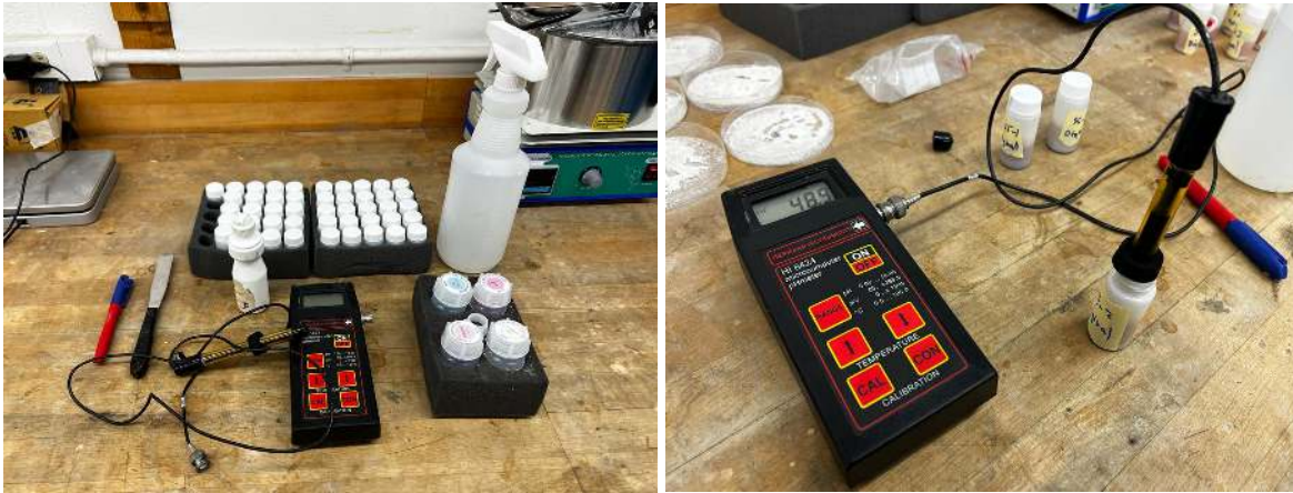
Figure 11 Rapid Chloride test setup and measurement
