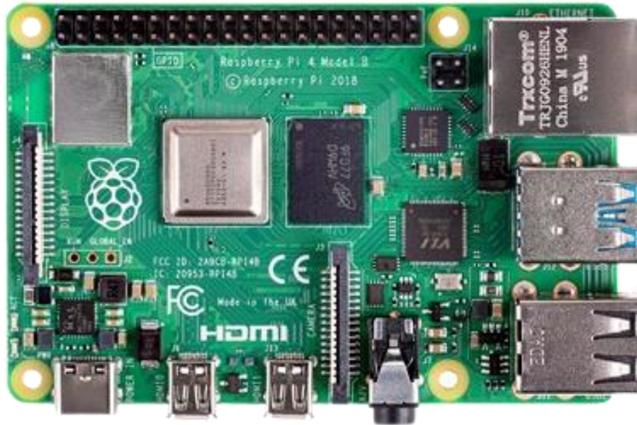
Figure 2.4: Top view of the Raspberry Pi 4 Model B, 8 GB RAM variant [89].
