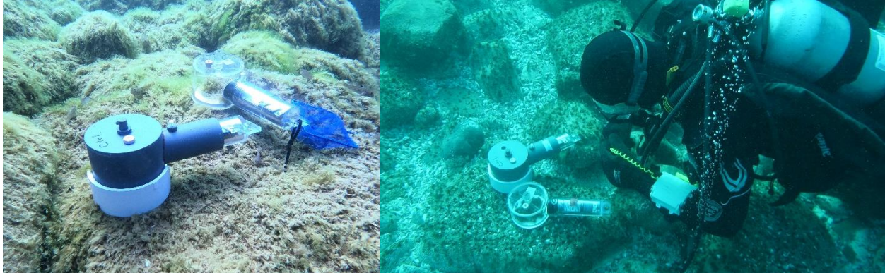
Figure 4. In situ incubations at Good Harbor Bay near Sleeping Bear Dunes National Lakeshore at a depth of 10 meters. We used pairs of light and dark benthic incubation chambers to measure the oxygen production and consumption by the benthic algae.
