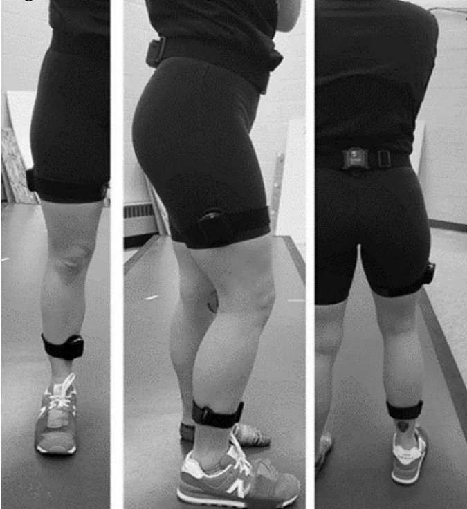
Figure 7. IMU Sensor placement
