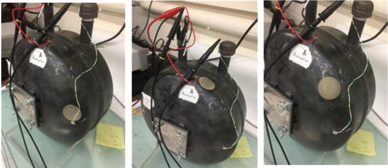
Figure 4.8: Large magnet positions on the structure. From left to right: in a middle distance between the actuator and sensor, near the sensor, and near the actuator.
