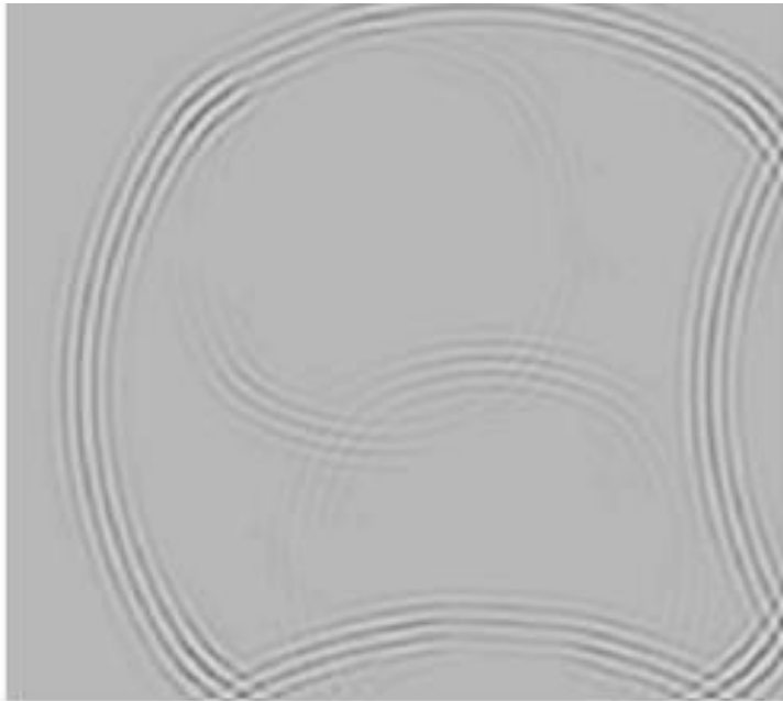
Figure 1.18 Propagating wave in composite plate at 0.21 milliseconds [30].
