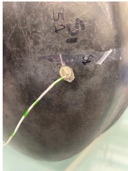
Figure 3.5: Additional close up view of another PZT mounted to tank.
