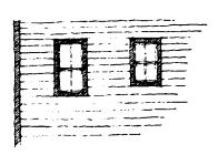
Heavy frames of wood, stone, or metal around windows and doors demonstrate good construction practice and the need for structural reinforcement. Thickened and protruding window sills help drain water away from openings, but, just as importantly, they help create an image of a well made and substantial building.
