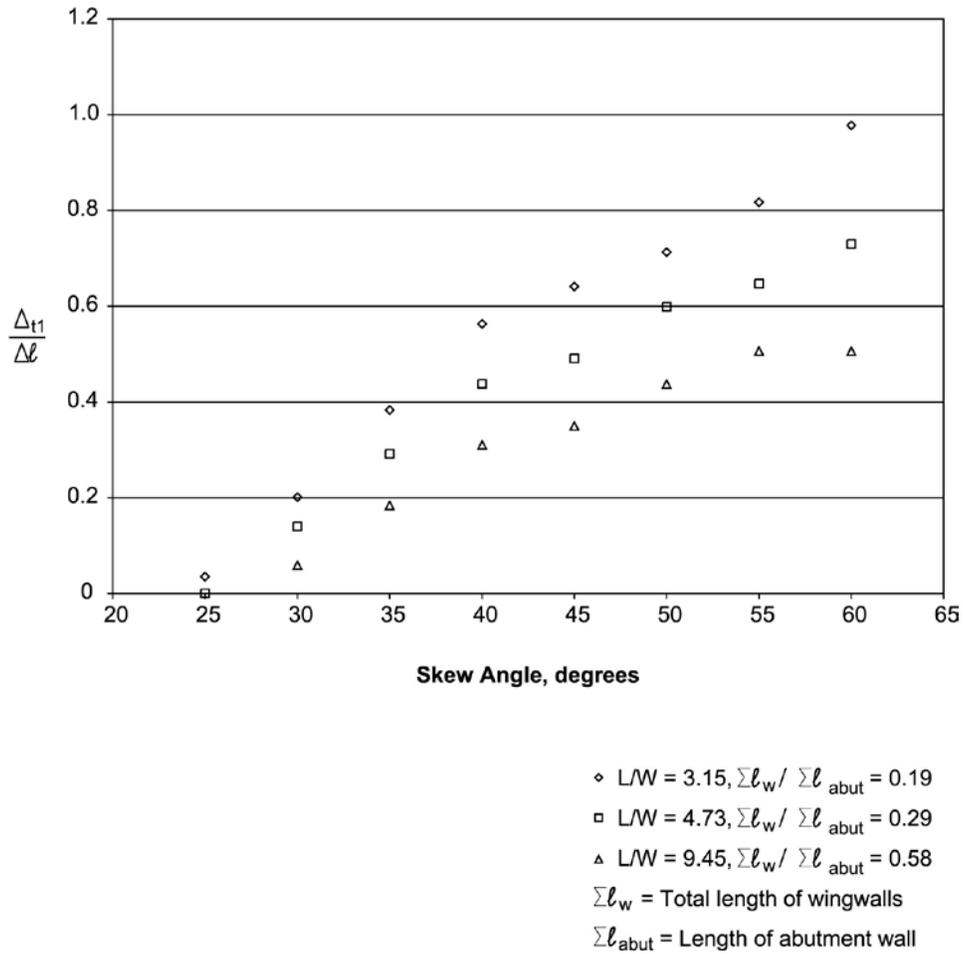
Figure 13. Relationship between transverse movement at the acute corner,  $\Delta_{t1}$ , and thermal expansion,  $\Delta l$ , for an expansion of 25.4 mm (1 inch) with constant-length bridge,  $L = 126.77$  m (415.92 ft), and varying  $L/W$ .
