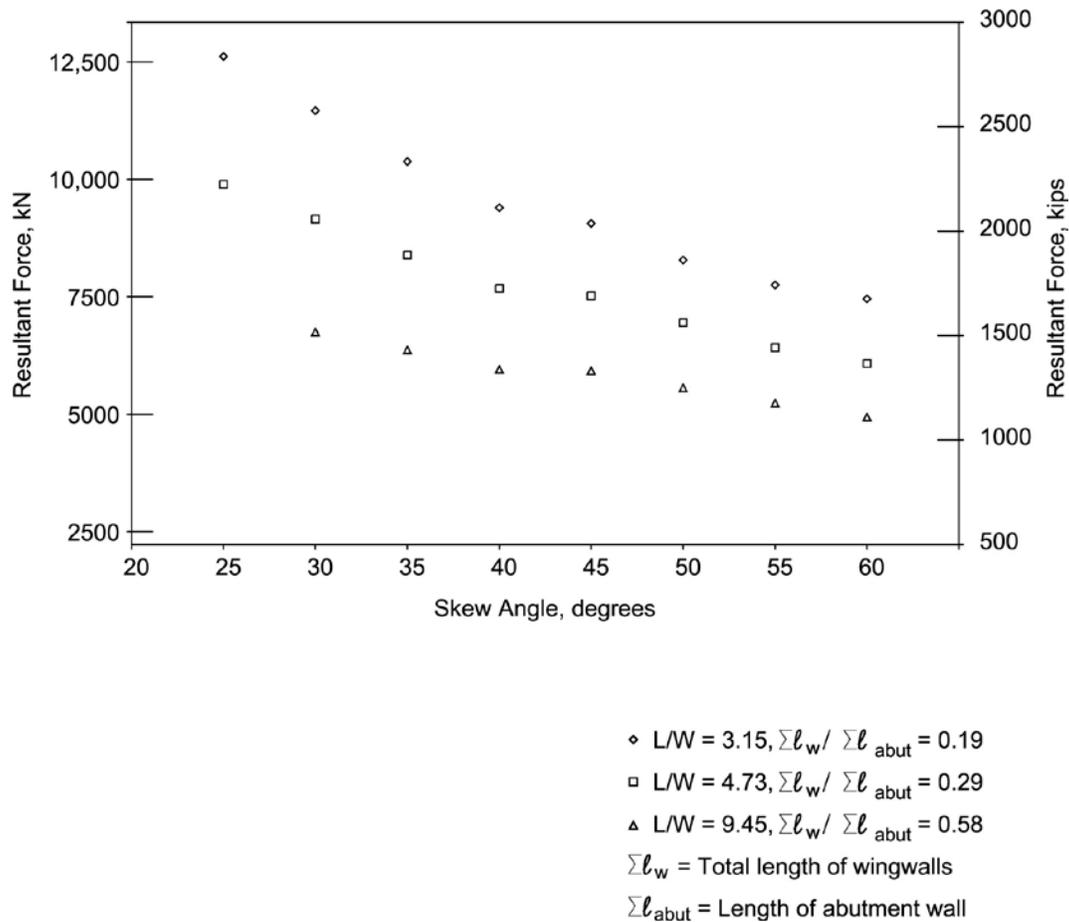
Figure 14. Relationship between resultant longitudinal restraint force and skew angle for thermal expansion,  $\Delta\ell$ , of 25.4 mm (1 inch) with constant-length bridge,  $L = 126.77$  m (415.92 ft), and varying  $L/W$ .
