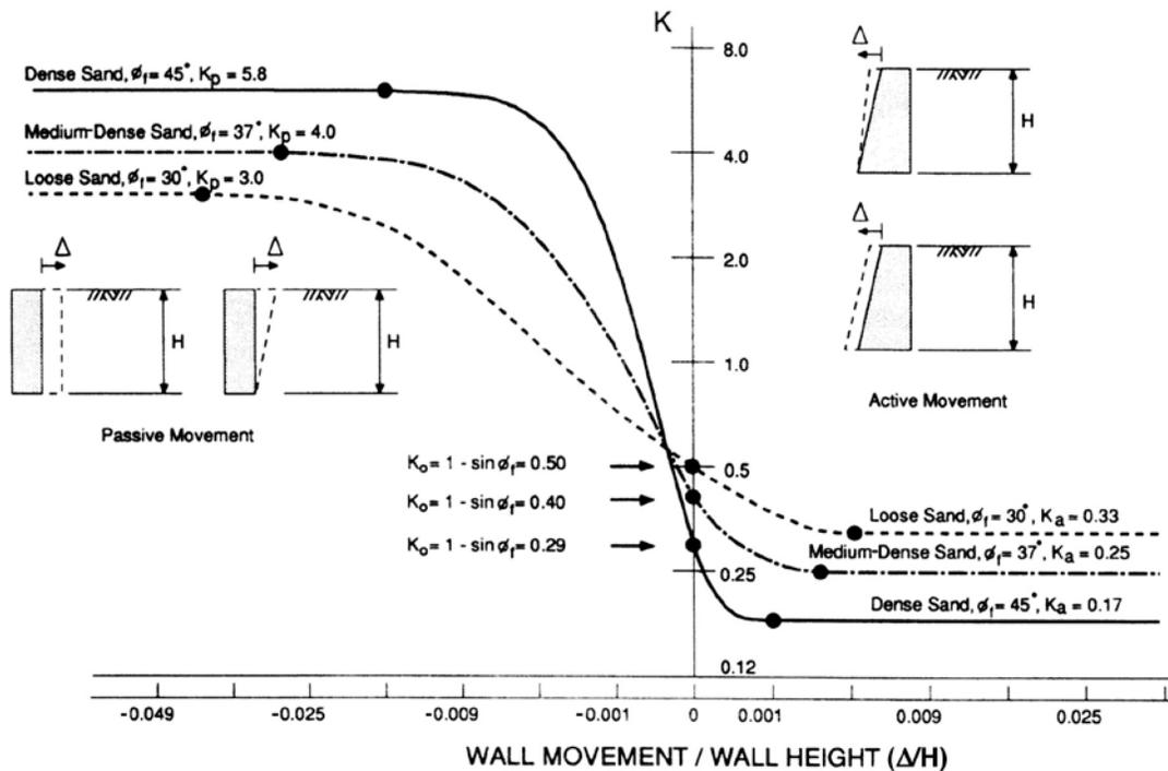
Figure 1. Relationship between abutment wall movement and earth pressure.<sup>(5,8)</sup>
